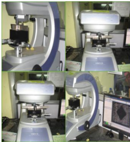
(a) Specimens positioned in Vickers hardness equipment.
