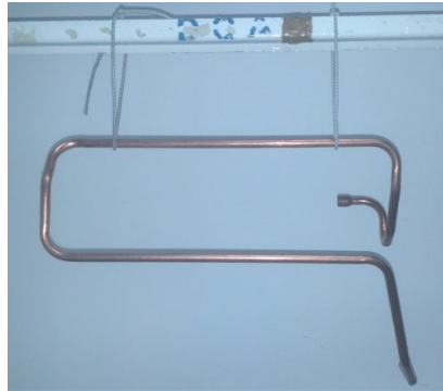
Fig. 6. Free-Free Test Setup of Copper Discharge Tube.
