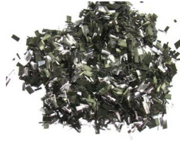
Fig. 1(b). Short Carbon Fiber (200 G.S.M., 5 mm Length).
