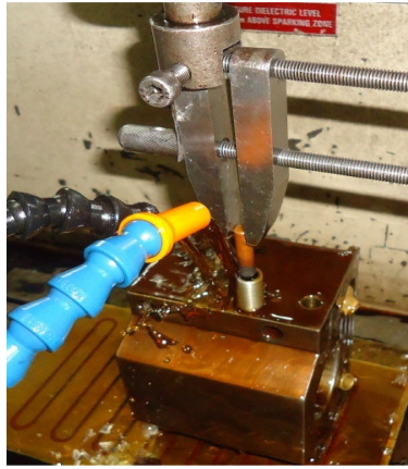
Fig. 1. Electronica-Small Die Sinking Electric Discharge Machine.
