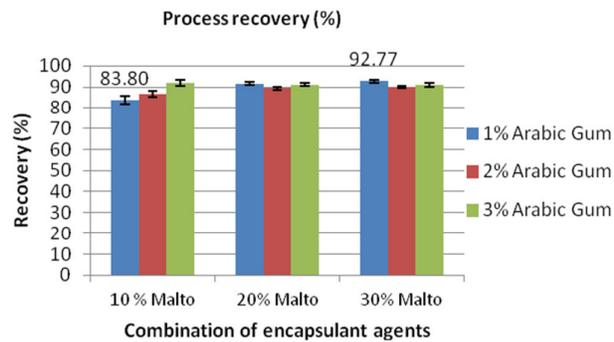
**Fig. 5. The Process Recovery (% , Per Mixture Weight) for Each Formulation of Spray Dried Vinegar.**
