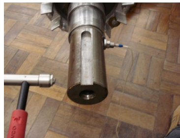
Fig. 6. Excitation and Measurement on the 250IVP Rotor.
