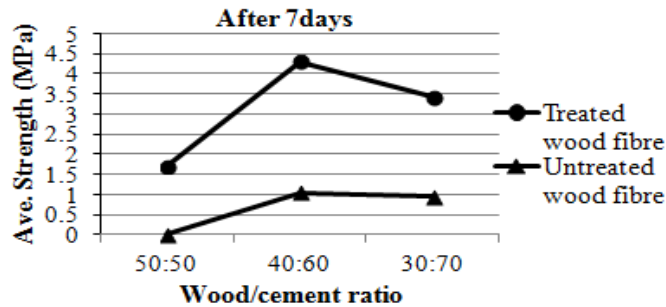
Fig. 5. Average Compressive Strength for Different Wood: Cement Ratio at 7 Days.
