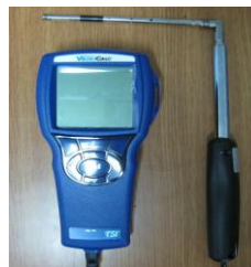
Fig. 2. Experimental Apparatus for Measuring Temperature and Velocity.
