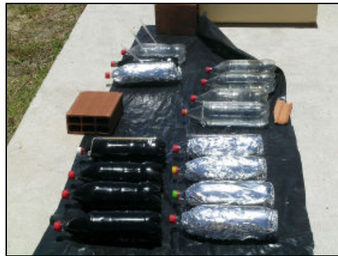
Fig. 2. In-progress Experiment Type I, in which Opaque, Transparent and Black Bottles were Displayed to the Sun.
