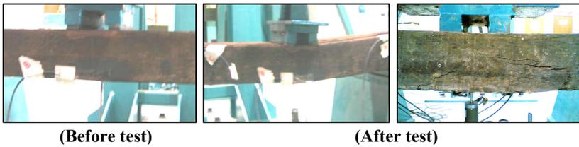
**Fig. 2. Crack Patterns for CPM2 – Longitudinal and Radial Crack.**
