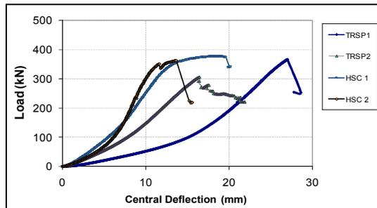
**Fig. 9. Comparative Response of Deflection at Rail Seat Positive Moment Test.**
