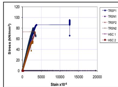
Fig. 11. Stress-Strain for TRSN and TRSP Sleeper at Rail Seat.
