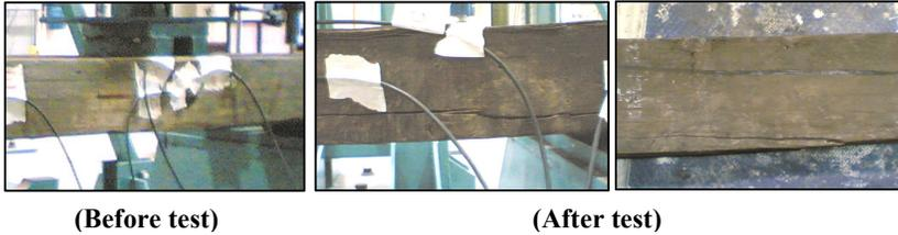
**Fig. 1. Crack Patterns for CPM1 – Longitudinal Crack.**
