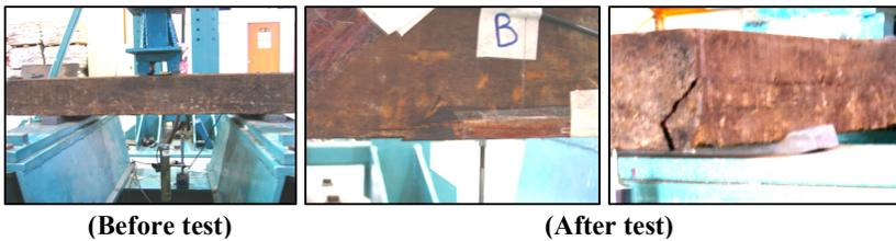
**Fig. 4. Crack Patterns for TRSP2 – Tangential and Longitudinal Crack.**
