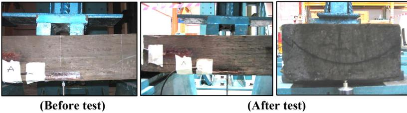
**Fig. 3. Crack Patterns for TRSP1- Tangential Crack.**
