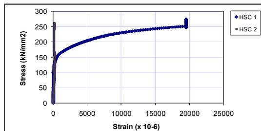
Fig. 12. Stress and Strain Relationship of High Strength Prestressed Concrete Sleeper at Rail Seat.
