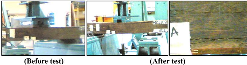
Fig. 5. Crack Patterns for TRSN1- Longitudinal Crack.
