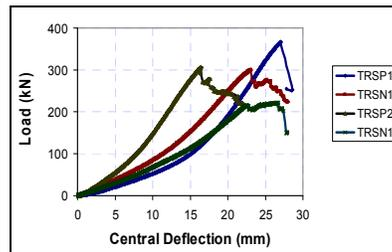
Fig. 8. Load-deflection of TRSN and TRSP Test.
