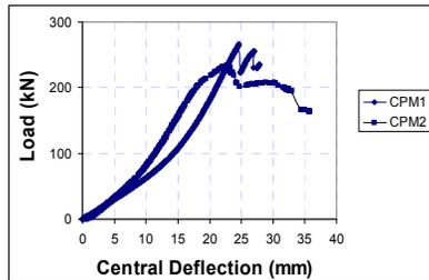
Fig. 7. Load-deflection of CPM Test.
