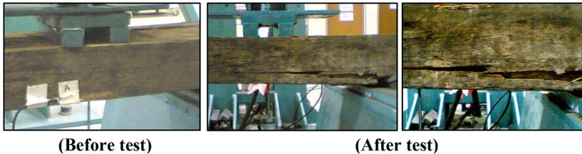
Fig. 6. Crack Patterns for TRSN2-Longitudinal Crack.
