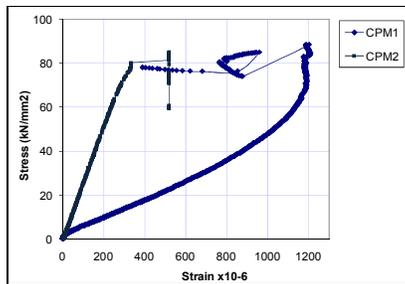
Fig. 10. Relationship of Stress and Strain for CPM Sleeper at Mid-span.
