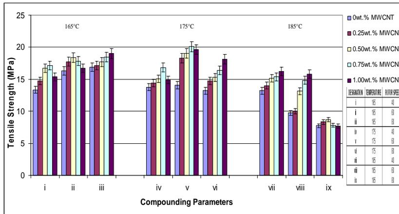
**Fig.3. Tensile Strength of PP-MWCNTs Composites Compounded at 165-185°C at Various Roller Rotor Speed of Internal Mixer.**
