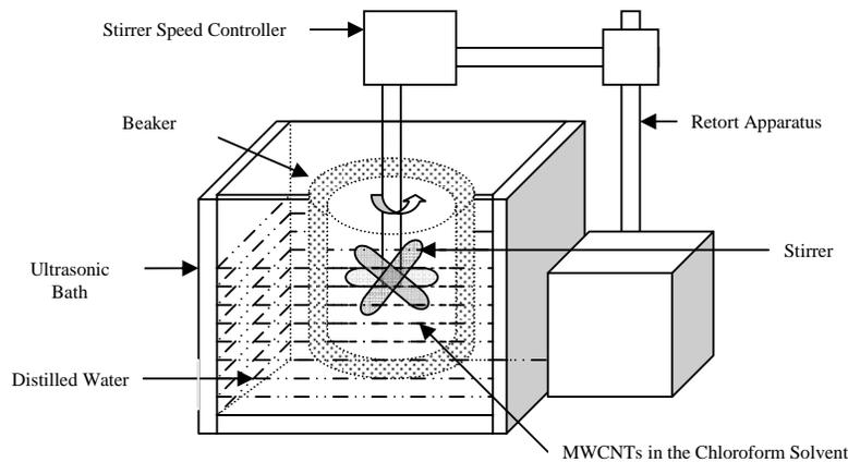
**Fig.1. Ultrasonication-Mechanical Stirrer Apparatus Set-Up for MWCNTs Dispersion Procedure.**
