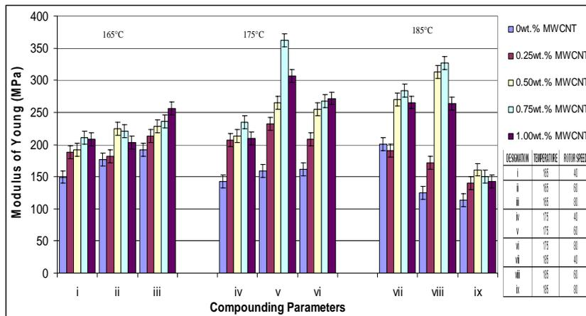
**Fig.4. Modulus of Young of PP-MWCNTs Composites Compounded at 165-185°C at Various Roller Rotor Speed of Internal Mixer.**
