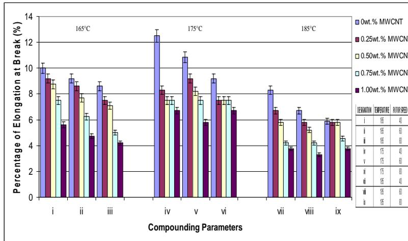
**Fig.5. Percentages of Elongation at Break of PP-MWCNTs Composites Compounded at 165-185°C at Various Roller Rotor Speed of Internal Mixer.**
