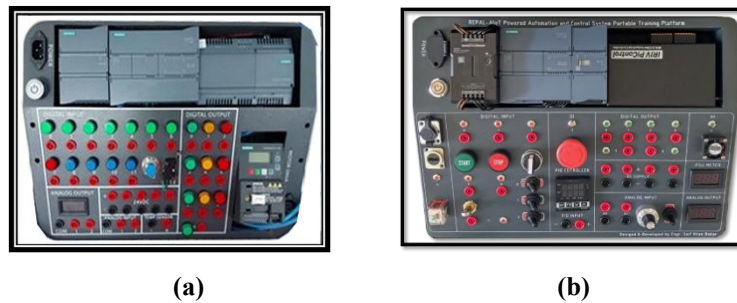
Fig. 2. Representative REPAL configurations: (a) VFD-based motor-control configuration and (b) PID temperature-control configuration.
