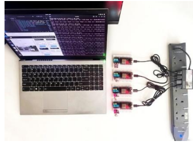
Fig. 7. The experimental setup of the GSU (MQ-4, MQ-136, MQ-137) and WSU, powered via a Type-C connection.
