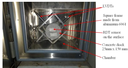
Fig. 6. Ohio CTE device.
