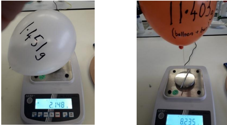
Fig. 2. Left, air filled balloon with 0.697 g weight increase due to balloon pressure. Right, Helium filled balloon with net negative weight of 3.168 g.
