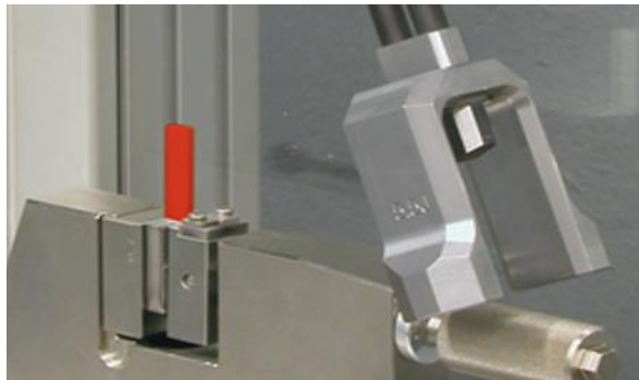
Fig. 5. Izod impact testing of polyurethane reinforced with nanosilica gel.
