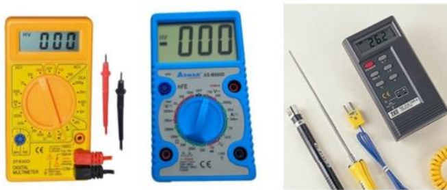
Fig. 8. Measurement instruments include of voltmeter, Ammeter, and thermometer reader.
