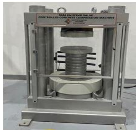
Fig. 4. Machine used for compressive strength test.
