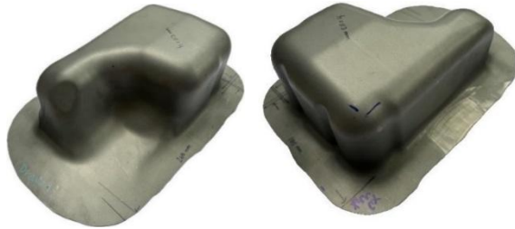
Fig. 25. The actual part after deep drawing process-01.
