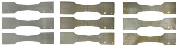
Fig. 4. Tensile test specimens in rolling direction of 0, 45 and 90 degrees, respectively.
