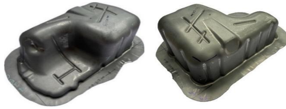
Fig. 27. Actual part after deep drawing process-02.
