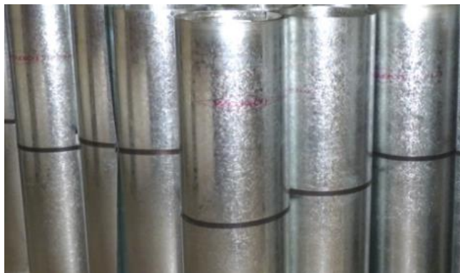
Fig. 3. 0.2 mm galvalume zinc plate.
