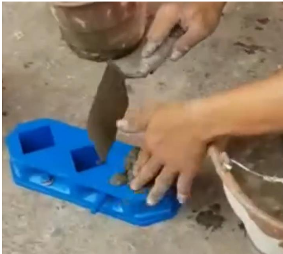
Fig. 7. Creation of mortar test specimens.
