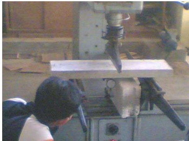
Fig. 13. Flexural testing of ferrocement.
