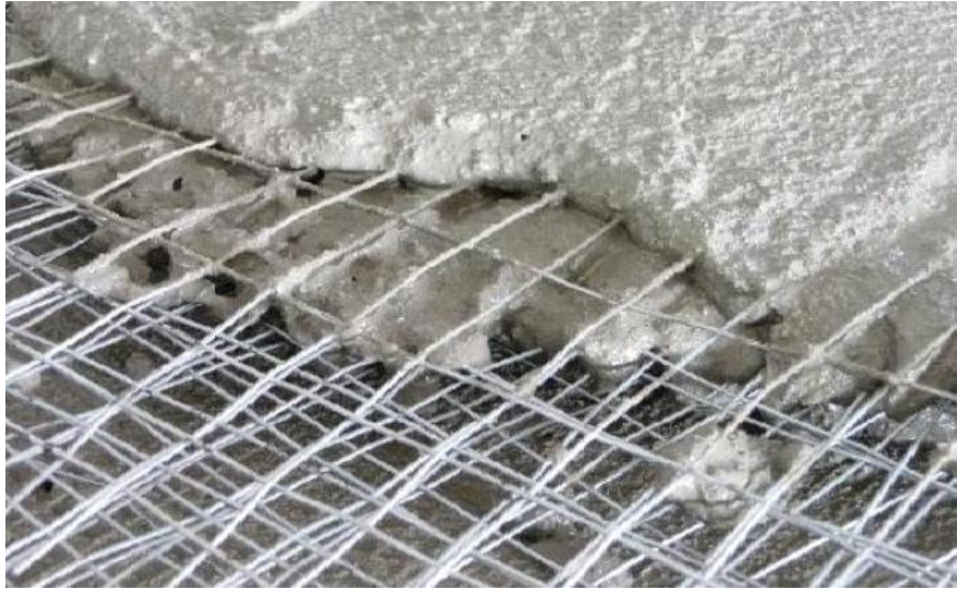
Fig. 1. Mortar and wire mesh as ferrocement components.
