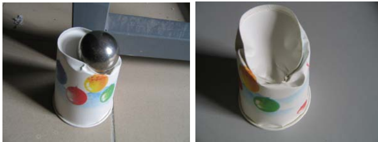
Fig.6. A Typical Shaped Cavity Generated in the Paper Cup Due to the Ball Impact.
