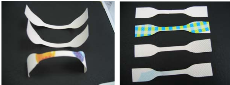
Fig.3. Specimens Obtained from the Paper Cups Before and After Testing.
