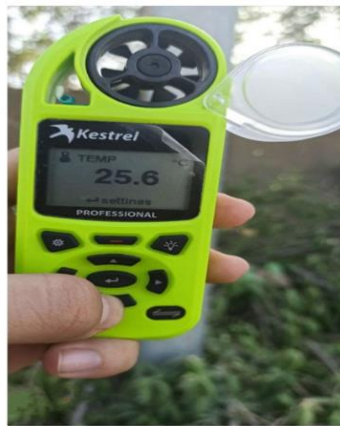
Fig. 6. An environmental meter device is called a Kestrel 5200 series hand-held device.
