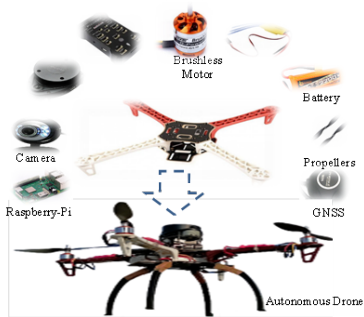
Fig. 4. Autonomous drone with object detection-ranging and navigation.
