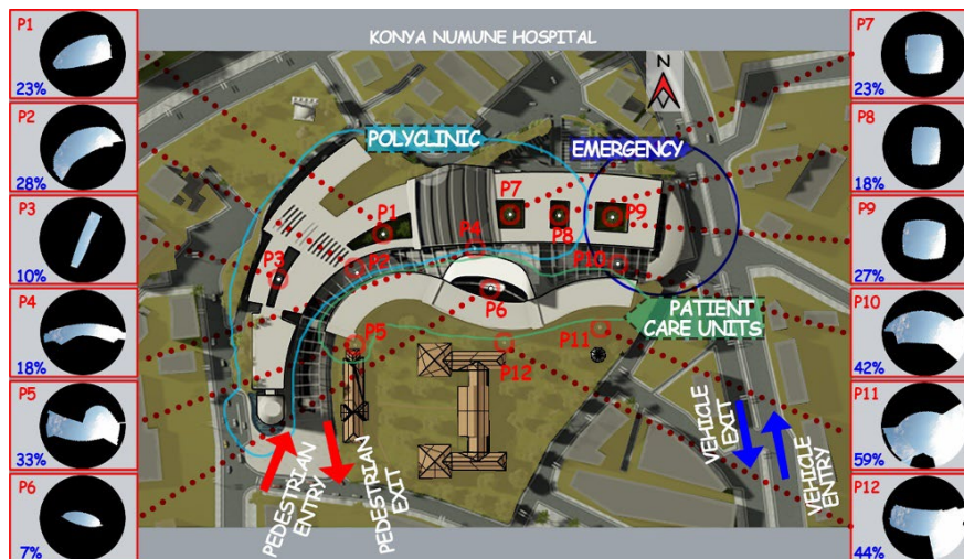
Fig. 8. SVF measurements observed at Konya Numune Hospital.
