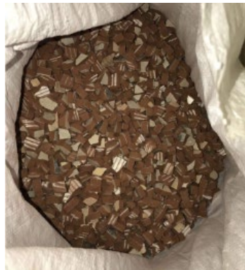
Fig. 1. Illustrative sample of crushed CTW aggregate used in this study.
