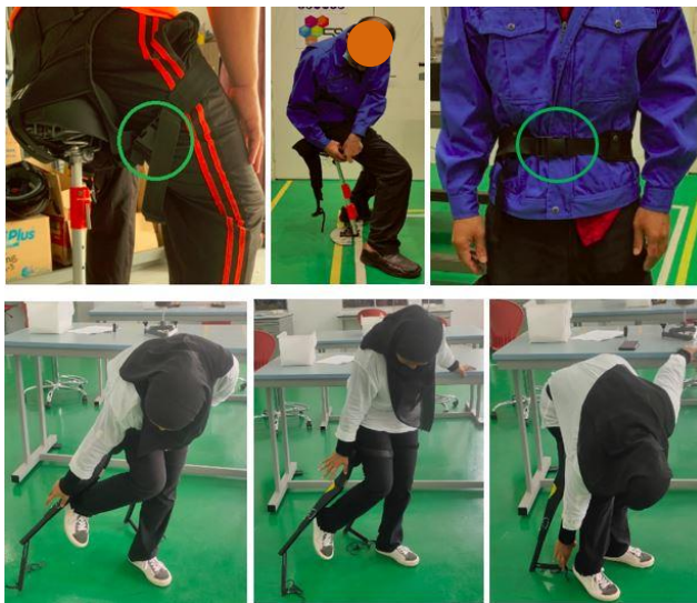
Fig. 9. Donning the single-stand chairless prototype exoskeleton (top) and double-stand chairless commercial exoskeleton (bottom).
