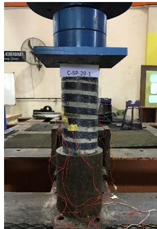
Partially confined column with CFRP
