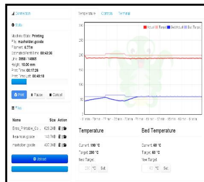
(a) Interface of OctoPrint temperature chart for measured and actual temperatures (bed and extruder).
