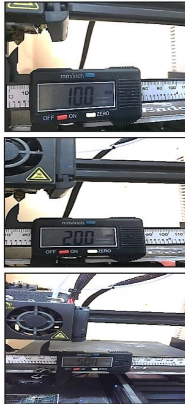
Fig. 9. 3D printer nozzle movement measurement.
