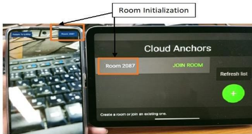
Fig. 8. The connection process between the host and client devices.
