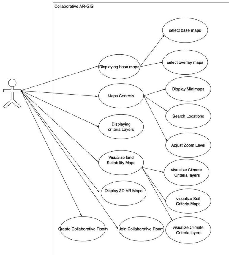
Fig. 6. The use-case of an AR-GIS prototype.
