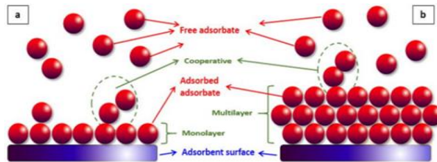
Fig. 1. Adsorption Models, Monolayer (a), and Multilayer (b)[11].
