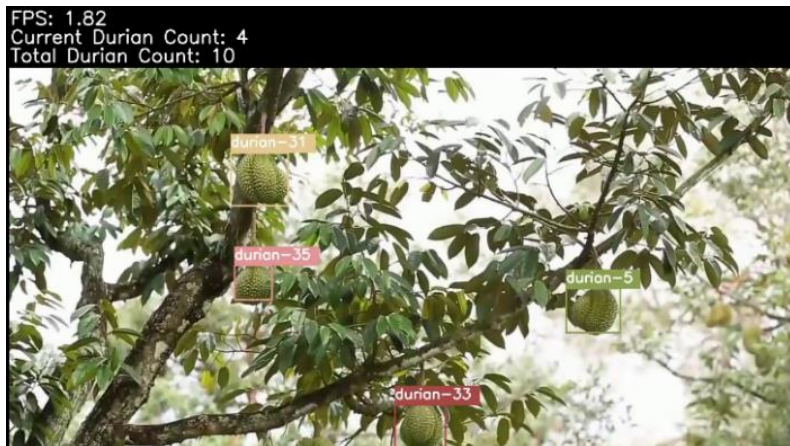
Fig. 4. Snapshot of the video inferencing results of the durian detection and counting system
