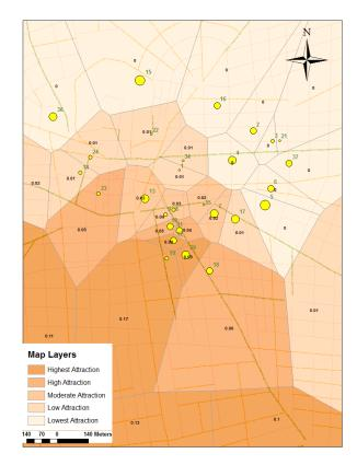
Fig. 10. The Gravity model applied on Thiessen polygons according to parking no.19 as drawn by ArcMap program (ArcGIS version 10.4.1).
