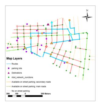
Fig. 13. Solving for alternative routes after adding road barriers (restrictions) as extracted from ArcMap program (ArcGIS version 10.4.1).
