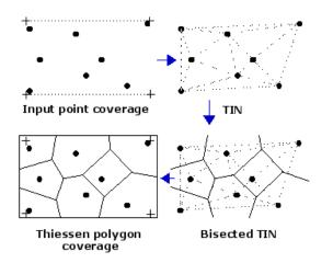
Fig. 7. Creating Thiessen polygon from points as extracted from ArcMap program (ArcGIS version 10.4.1).
