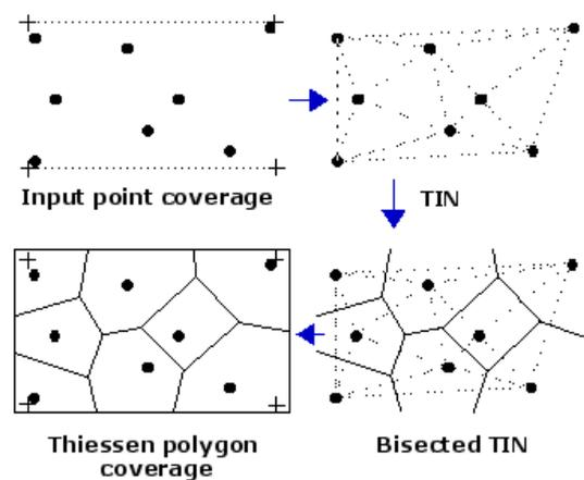
**Fig. 7. Creating Thiessen polygon from points as extracted from ArcMap program (ArcGIS version 10.4.1).**
