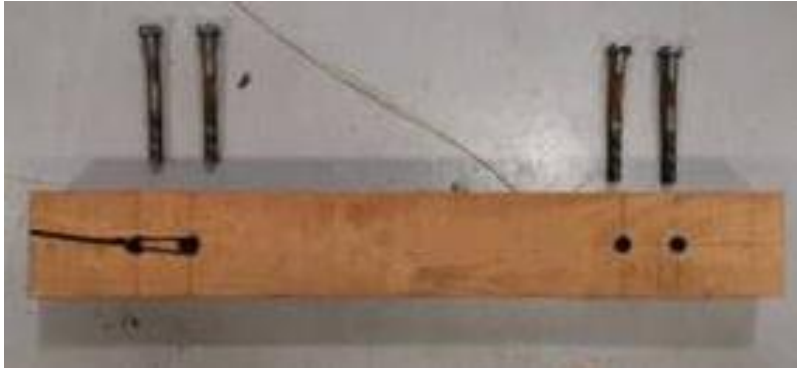
Fig. 3. Bolted connection specimen with s_b = 50 mm and e_t = 100 mm.
