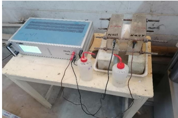
Fig. 3. The rapid chloride penetration test (RCPT) measurement device.
