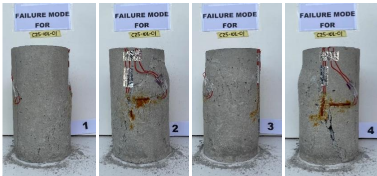
Fig. 4(b). Modes of failure of HSPF confined concrete specimens at 4 different angles, after taking off the confined plastic film.
