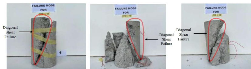
Fig. 3. Failure modes of unconfined concrete specimens.
