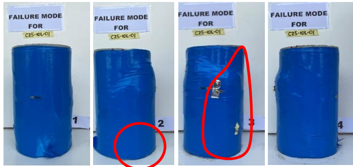
Fig. 4(a). Modes of failure of HSPF confined concrete specimens at 4 different angles.
