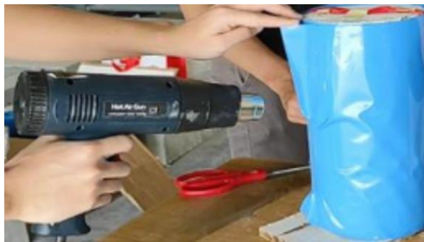
Fig. 1. Heat blow of 105 °C on HSPC confined concrete.
