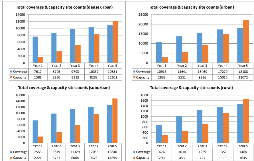
Fig. 5. Total site counts estimated by the 5G-RAND tool over a 5-year period.
