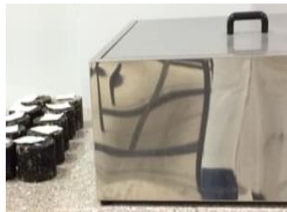
(b) Put the mixtures in water bath at 60°C.
