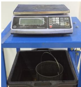
(a) Test the mixture for bulk specific gravity of specimen ( G_{mb} ).
