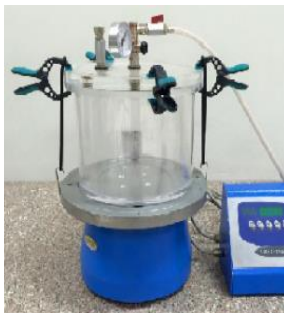
(c) Tested the mixture for maximum specific gravity of specimen ( G_{mm} )
