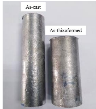
Fig. 3. Composite billet before and after thixoforming process.
