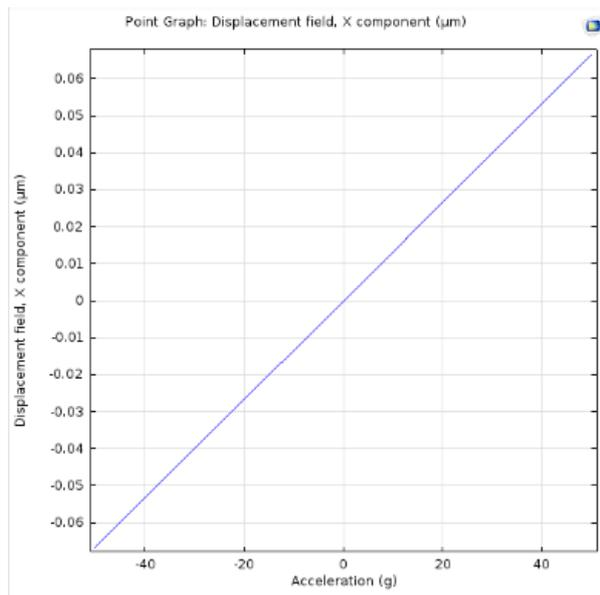
**Fig. 9. Displacement versus acceleration graph for polysilicon**
