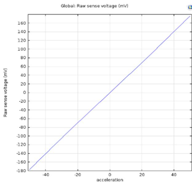
**Fig. 11. Voltage versus acceleration graph for germanium.**
