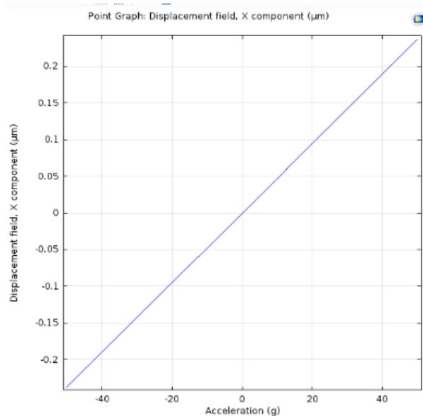
**Fig. 10. Displacement versus Acceleration graph for germanium.**
