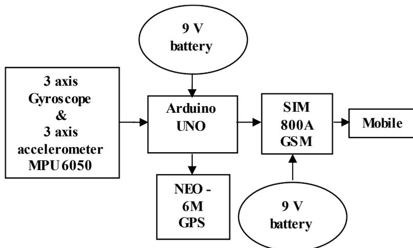
**Fig. 1. Block diagram of road monitoring system architecture.**
