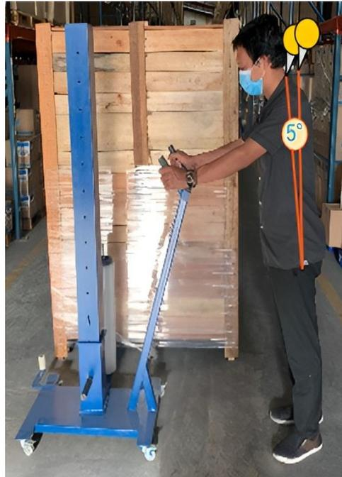
Fig. 15. Usage of wrapping trolley.
