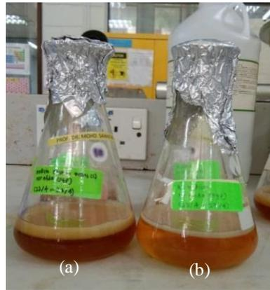
**Fig. 4. Biocellulose pellicle from the fermentation in (a) pineapple peel extract and (b) HS medium.**
