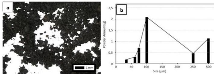
**Fig. 2. Photograph image of carbon particles (a) and their particle size distribution (b).**
