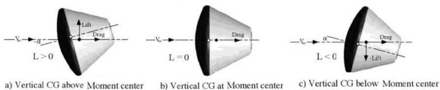
**Fig. 1. Apollo with different angles of attack.**
