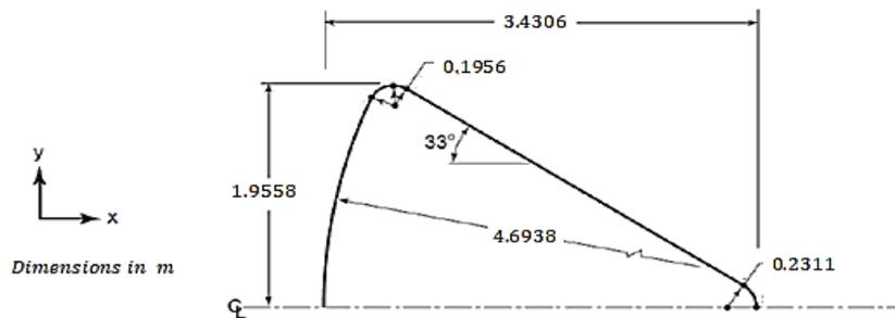
Fig. 3. Schematic representation of Apollo model AS-202 [19].
