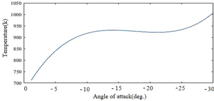
**Fig. 9. Temperature distribution at Mach 6 and different values of attack angle.**
