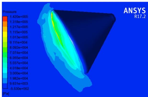
**Fig. 10. Variation of pressure contour for Apollo at Mach 10 and AoA = -30°.**
