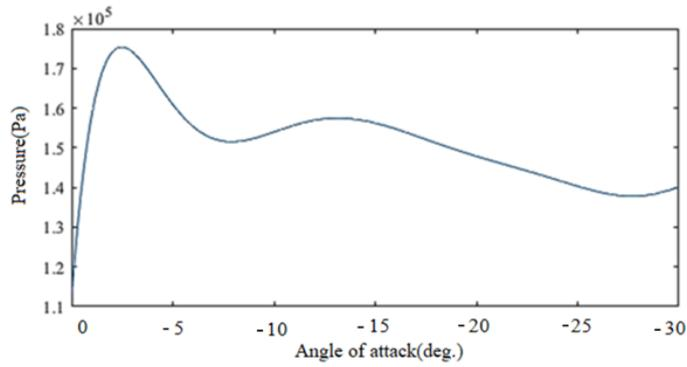
**Fig. 11.** Pressure distribution at Mach 6 and different values of attack angle.
