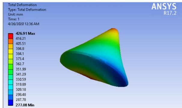
**Fig. 12.** Variation of deformation contour for Apollo at Mach 10 and AoA = -30°.
