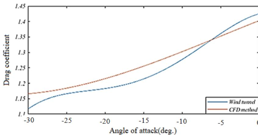
Fig. 5. Drag coefficient with varies the angle of attack at Mach 5 and  $Re = 7 \times 10^5$ .
