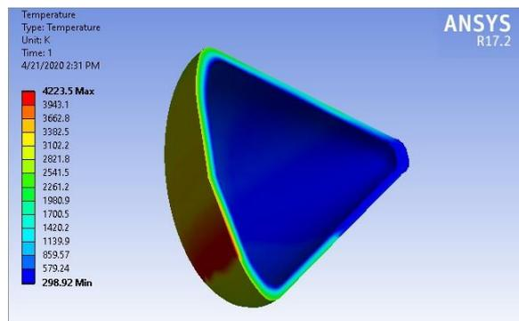
**Fig. 8. Temperature distribution over the thickness of the Apollo model at Mach 10 and AoA=-30°.**
