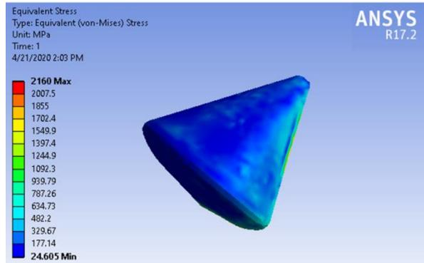
Fig. 14. Variation of stress contour for Apollo at Mach 10 and AoA =-30°.
