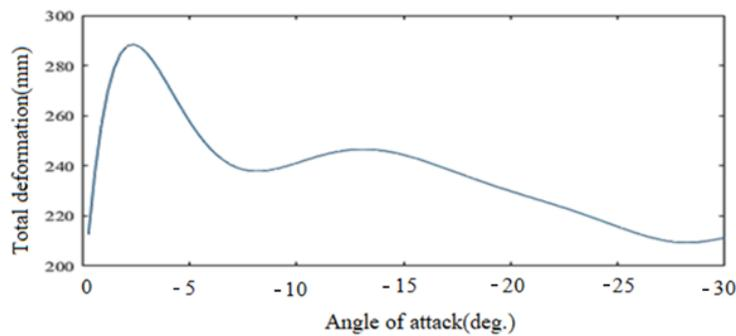
**Fig. 13.** Total deformation over the Apollo for different values of attack angle at Mach 6.
