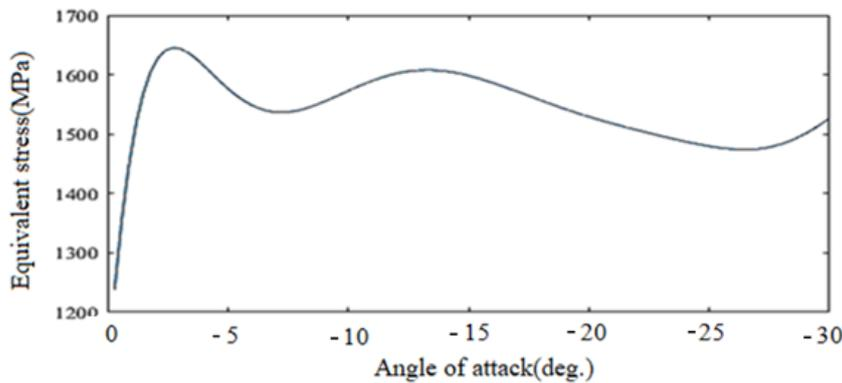
Fig. 15. Stress distribution over the Apollo for different values of attack angle at Mach 6.
