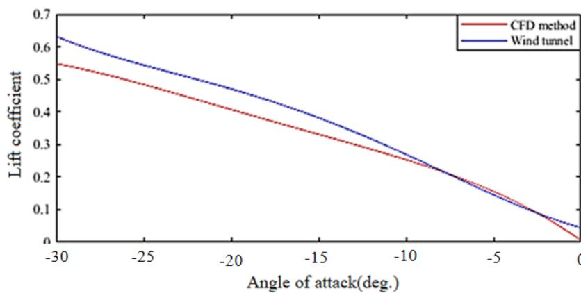
Fig.6. Lift coefficient with varies the angle of attack at Mach 5 and  $Re = 7 \times 10^5$ .
