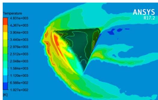
**Fig. 7. Variation of temperature contour for the Apollo at Mach 10 and AoA=-30°.**
