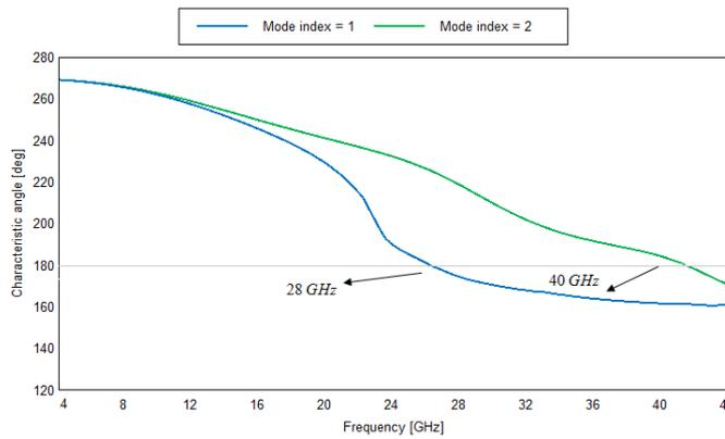
**Fig. 15. Characteristic angles of modes 1-2 of the bowtie antenna.**
