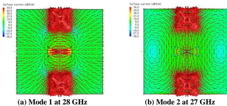
**Fig. 20. Current distribution of the MTM bowtie antenna**
