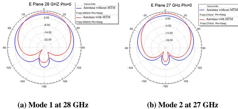
**Fig. 23. Radiation Pattern of Bowtie antenna with and without MTM- E Plane**
