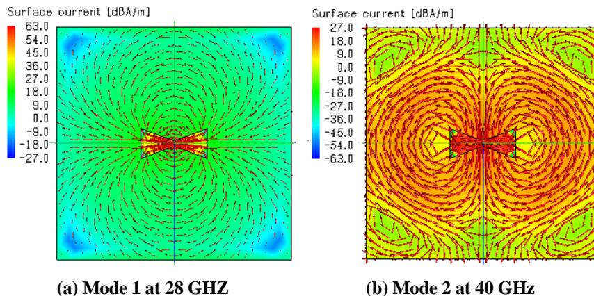
**Fig. 17. Current distribution on the bowtie antenna.**
