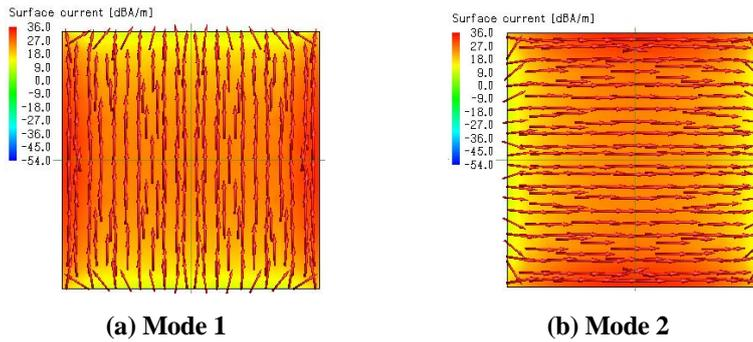
**Fig. 14. Current distribution of the first two modes on the ground plane at 28 GHz**
