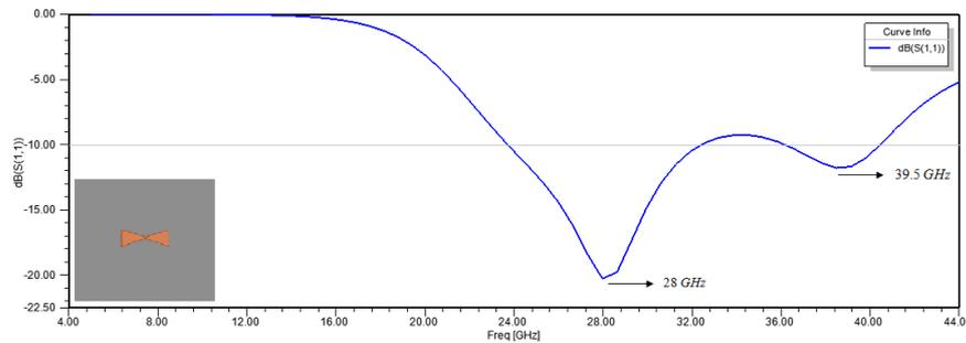
Fig. 2. The reflection coefficient S(1,1) of the bowtie antenna.
