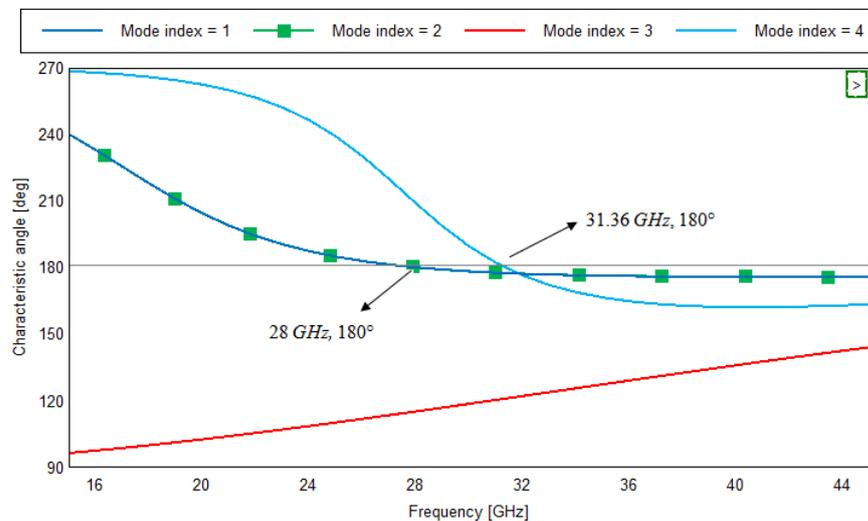
Fig. 12. Characteristic angles of modes 1-4 of the ground plane.
