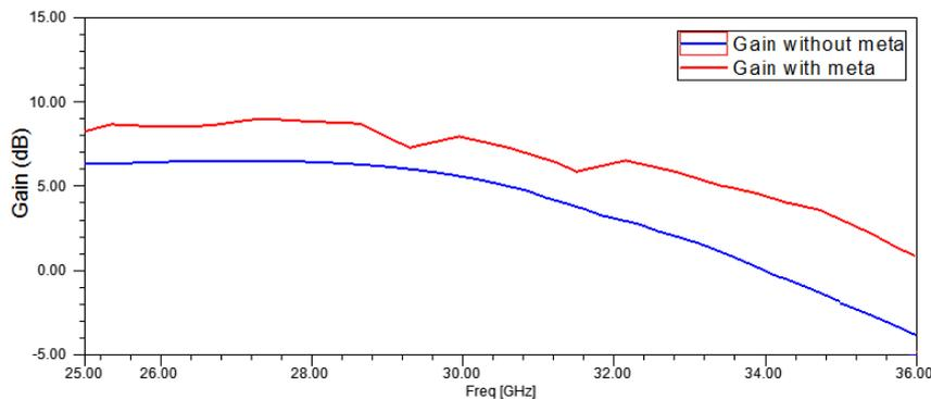
**Fig. 22. The gain vs frequency of the bowtie antenna with and without MTM unit cells.**
