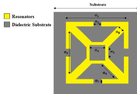
Fig. 3. The geometry of the MTM Unit Cell (Front View).
