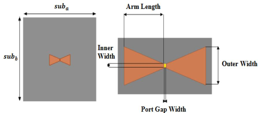
Fig. 1. Bowtie antenna geometry (Front View).
