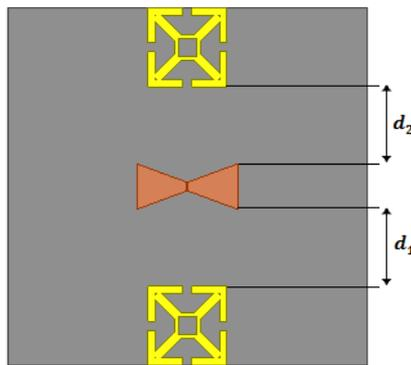
**Fig. 10. Geometry of MTM antenna (Front View).**
