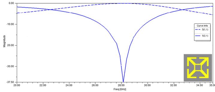
**Fig. 4. The reflection coefficient S(1,1) of the MTM unit cell.**
