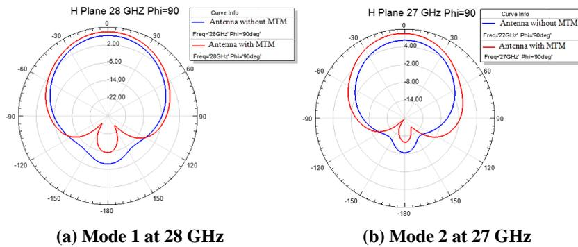
**Fig. 24. Radiation pattern of Bowtie antenna with and without MTM- H plane.**
