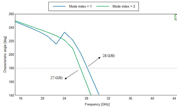
**Fig. 18. Characteristic angles of modes 1-2 of the MTM bowtie antenna.**
