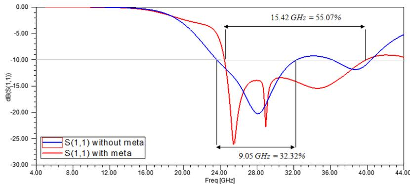
**Fig. 21. The reflection coefficient  $S(1,1)$  of the Bowtie antenna with and without MTM unit cells.**
