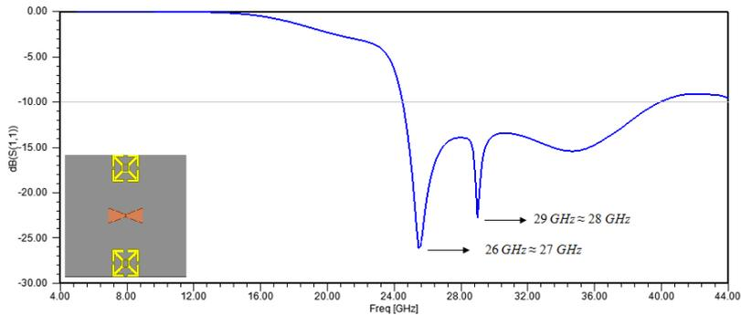
**Fig. 11. The reflection coefficient S(1,1) of the MTM bowtie antenna.**
