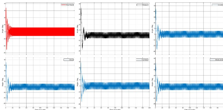
**Fig. 6. The roll angle simulation results of six surface vessels at a high damping ratio and sea state of 7 (wave height of 9.0 meters).**
