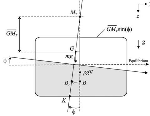
**Fig. 3. Transverse metacentric stability. Reprinted from [21].**
