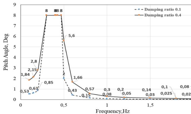
**Fig. 8. The Pitch angle profile of all six surface vessels at different damping ratios and encounter wave frequencies.**
