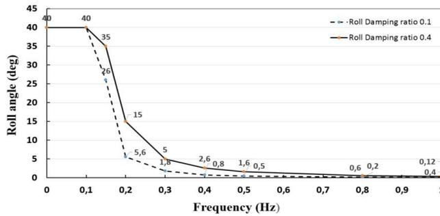
**Fig. 7. The Roll angle profile of all six surface vessels at different damping ratios and encounter wave frequencies.**
