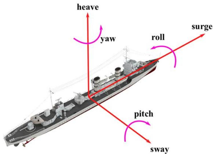
Fig. 1. Six motions of a destroyer.
