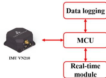
Fig. 9. The connection diagram of the motion data logging device
