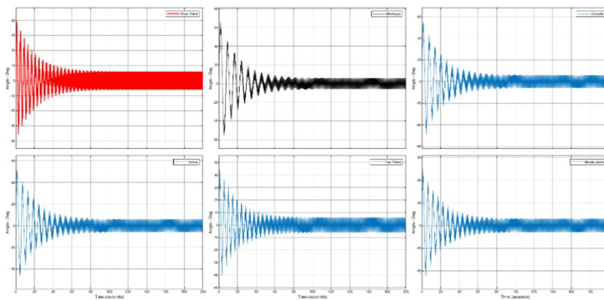
**Fig. 5. The Roll angle simulation results of six surface vessels at a low damping ratio and sea state of 7 (wave height of 9.0 meters).**
