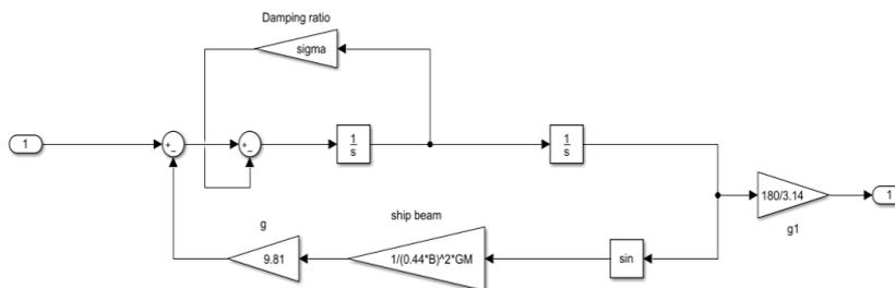
Fig. 4. The Simulink model to estimate the response of the ship.
