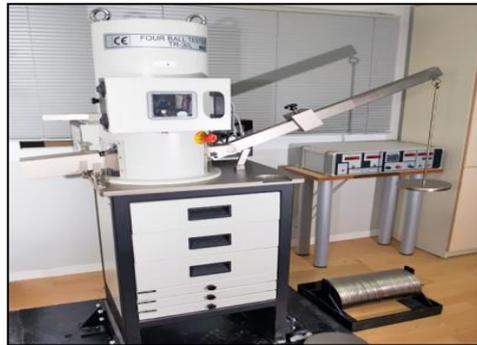
Fig. 1. Photograph of the wear testing machine.
