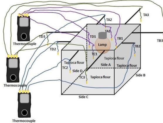
**Fig. 4. The 3D layout of the heat transfer toolbox.**
