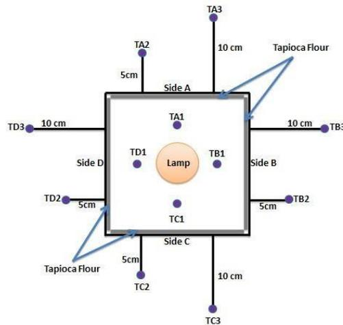
**Fig. 3. The 2D layout of the heat transfer toolbox (taken from the top of the box).**
