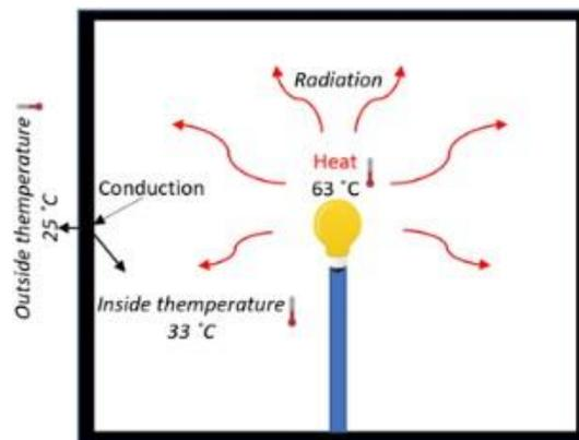
**Fig. 2. Illustration of the concept of the equipment used for heat radiation.**
