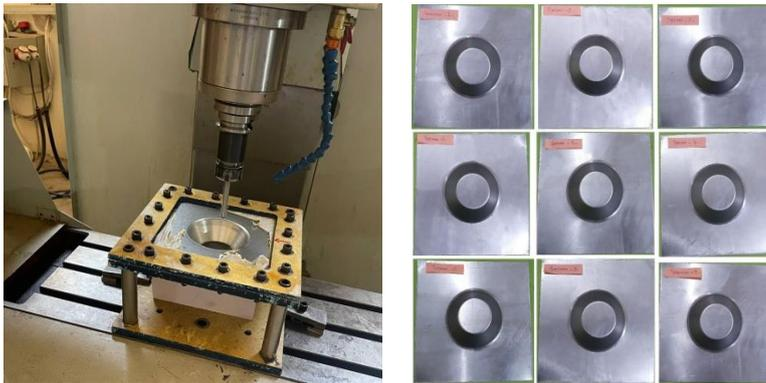
**Fig. 4. Various views of the cups produced (a) TPIF process (b) Produced cylindrical cups.**
