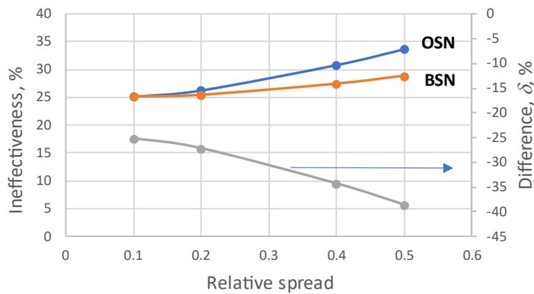
**Fig. 7. Results of heat exchanger ineffectiveness with OSN and BSN nonuniform flow profile generated with B(1.1, 1.1) for NTU = 3.0 and  $C_r = 1.0$ . Data is read from the original graph published in [28].**
