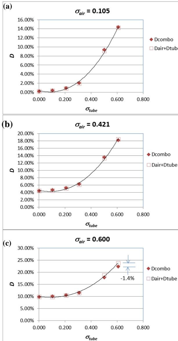
Fig. 3. Variation of  $D$  vs. standard deviation (Skew of both fluid sides = 0.00).
