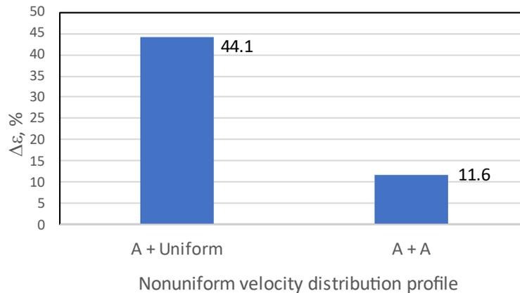
**Fig. 8. Results of effectiveness degradation rate for (a) Configuration A and Uniform, (b) two-sided Configuration A, (A + A). Flow in counter-flow arrangement with  $Re = 100,000$  to  $600,000$ . [16].**
