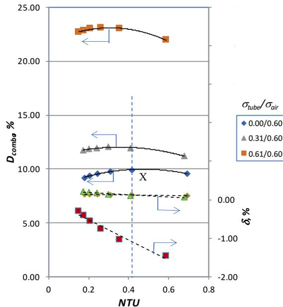
**Fig. 5. Plot of  $D_{combo}$  and  $\delta$  vs.  $NTU$  at specific air-side and tube-side standard deviations ( $N_i = 0.41$ , skew = 0.00).**
