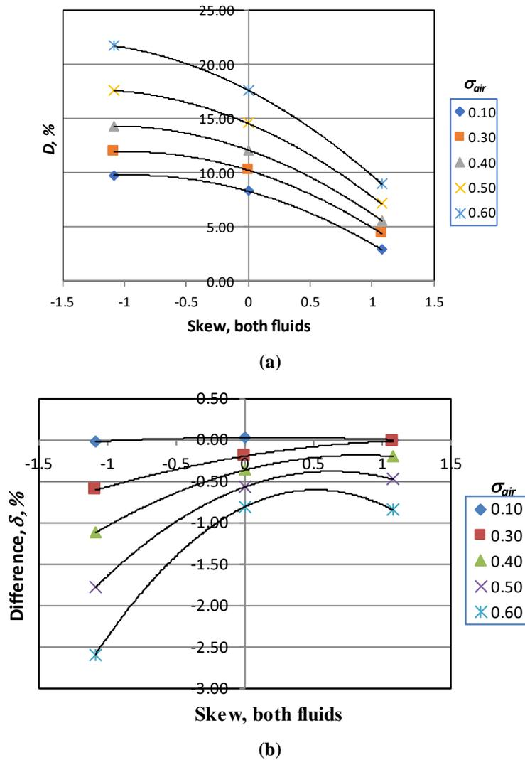
**Fig. 4. (a)  $D_{combo}$ , % (b) Difference  $\delta$  vs. with the same skew on both fluid sides ( $\sigma_{tube} \sim 0.46$ ).**
