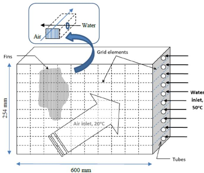
**Fig. 2. Numerical model of fin-tube heat exchange. Inset: Zoom-in view of a discrete element showing the crossflow arrangement of air and water.**
