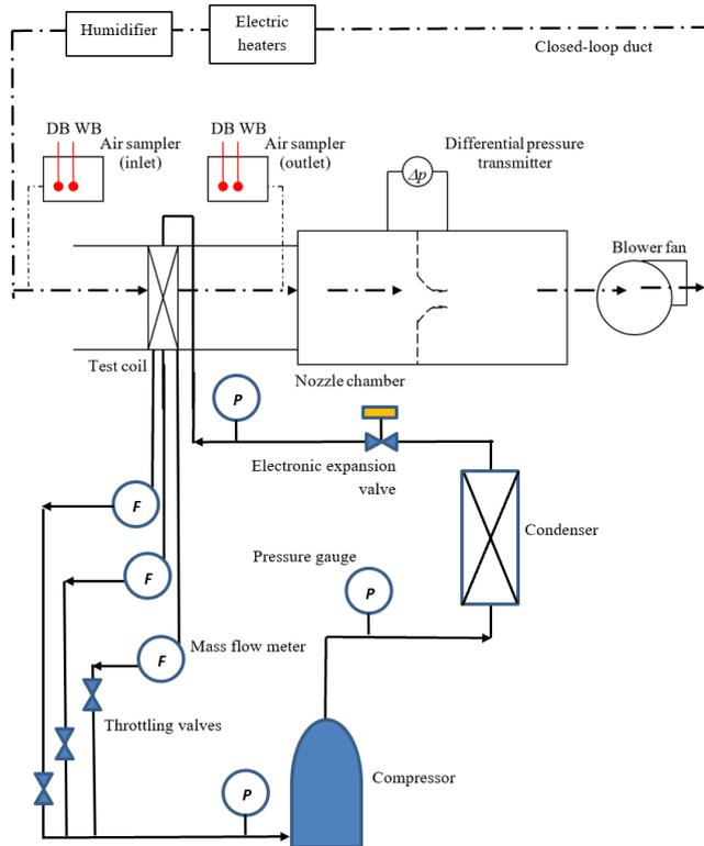
Fig. 9. Schematic diagram of test rig (simplified).
