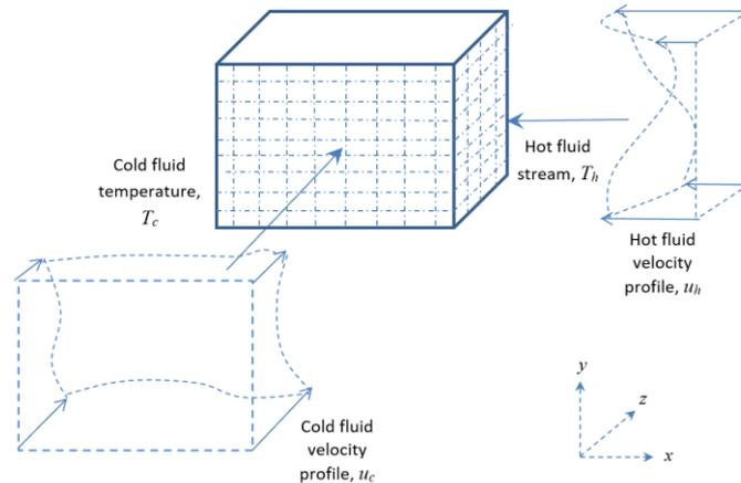
**Fig. 1. Illustration of heat exchanger.**
