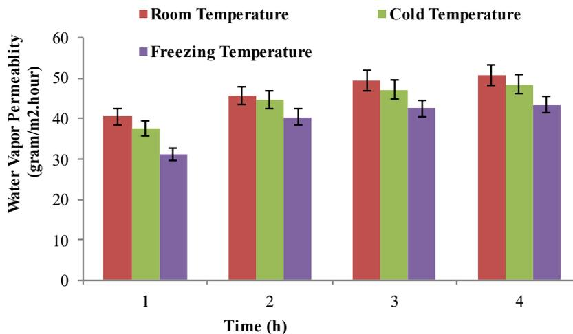
**Fig. 6. The effect of storage at various temperature on water vapor permeability of bioplastic.**
