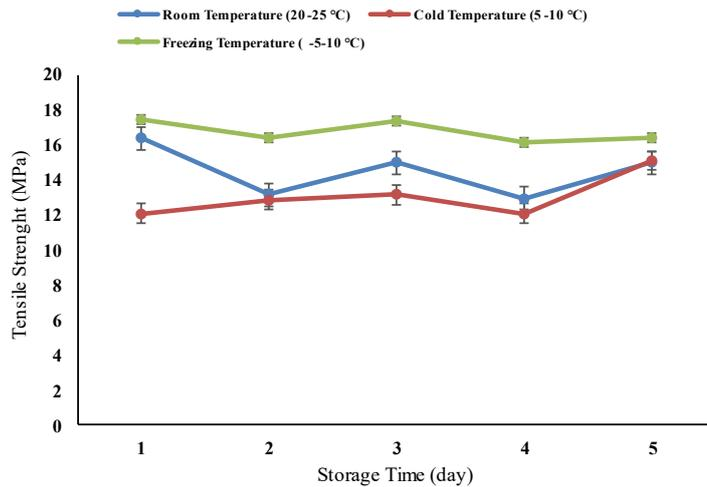
Fig. 3. The effect of storage at various temperature on tensile strength corn starch-based bioplastic with NFC as filler.
