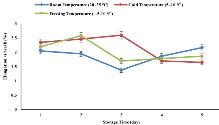
Fig. 4. The effect of storage at various temperature on elongation at break corn starch-based bioplastic with NFC as filler.
