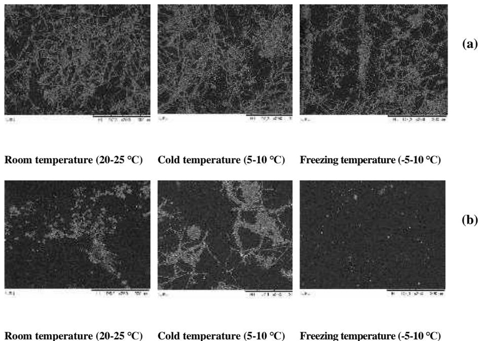
**Fig. 5. Morphology of surface bioplastic at various storage temperature using scanning electron microscope (SEM) with magnification 250× (a) Before storage (0 day) and (b) after day-5.**
