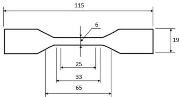
**Fig. 2. Geometry and dimension tensile strength test specimen of bioplastic (unit in mm) [13].**
